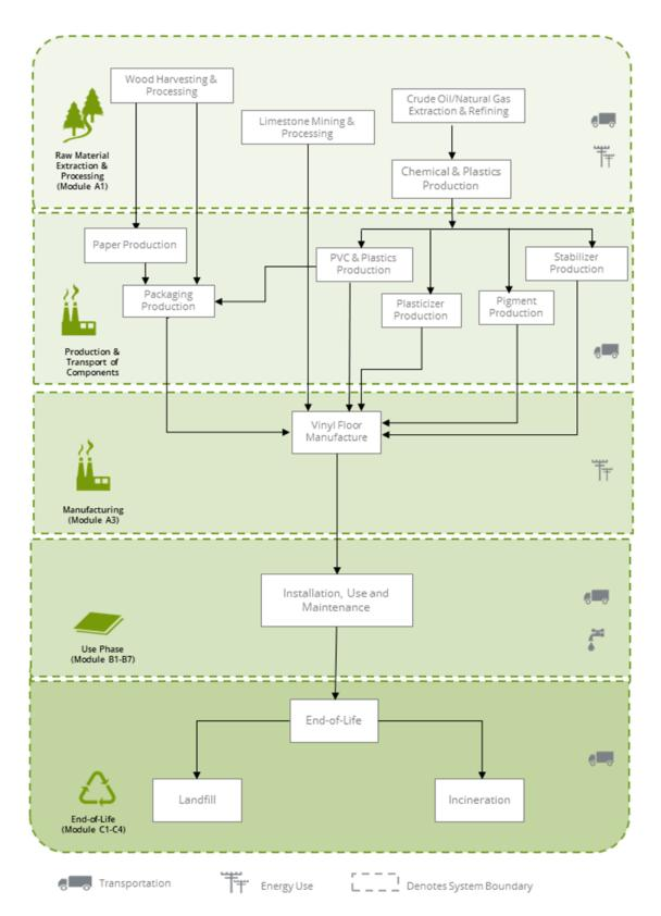
**Figure 1.** Flow Diagram for the life cycle of the Rigid Click product system.
