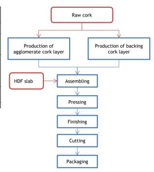
The production process begins with the manufacturing of agglomerate pressed cork and backing layer. Following this process, HDF is assembled to both cork layers. This stage is followed by printing. After printing, the product is assembled to a PVC layer, and then undergoes trough a pressing process. The top layer is coated with a protective varnish, creating a hard wearing surface. The next stage consists in pre-cutting and cutting, in order to shape the planks. The last stage is packaging.
