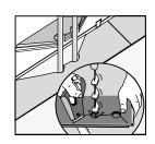
Cut the plank with a 45° angle towards the hole. The cut-off piece is glued in the position again. Cover the hole with a pipe sleeve.
