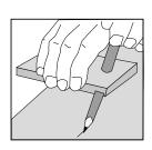
Transfer the shape of the wall to the planks. Do not forget to allow 5mm(0.2") for the expansion gap.
