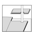
Drill the required holes in the planks, making a hole on the plank 10mm (0.4") bigger than the pipe diameter.
